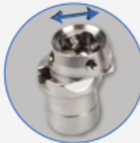
Offering a tube-clamp adapter on one end, the 3T85 adapter slides in either direction allowing for custom lateral offset. Safety-locked from completely sliding apart, a single screw sets offset distance.\* Our new Arch Slide Adapter (T6E87) uses an arched dovetail slide to allow adjustable angles, increasing lateral offset capability based on the pylon length. Use when more than 11mm lateral offset is needed.
