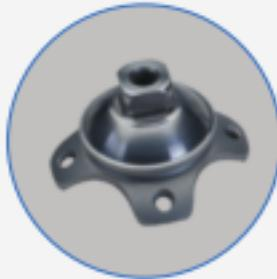
Connector between Socket and Pylon (Lamination). Rough-machined prongs for improved lamination bonding. Includes rubber lamination dummy. (Not included in weight) 8.2 mm center hole.
