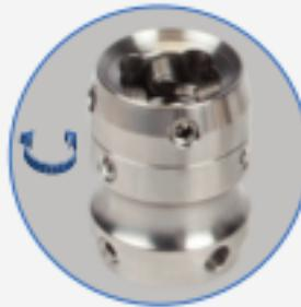
Created for use when distance is a problem and conventional double head adapters do not solve issues requiring rotation of components. Now, to modify the angle of the socket and pylon, this double-head receiver rotates to make final adjustments for correct toe out and knee directions. Easy-access set screws lock the adapter at desired position.
