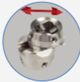
With receivers on both ends, this adapter slides in either direction to create a custom lateral offset. Safety-locked from completely sliding apart, a single screw sets offset distance. Our new Arch Slide Adapter (T6E98) uses an arched dovetail slide to allow adjustable angles, increasing lateral offset capability based on the pylon length. Use when more than 11mm lateral offset is needed.
